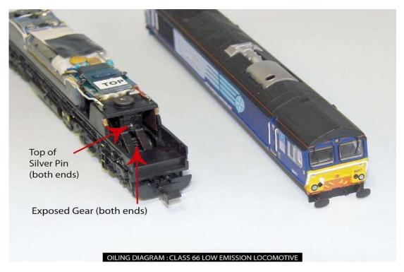
Please note that oiling these points is suggested as an 'extra' to oiling the gears in the locomotive instructions and not as an alternative to.
